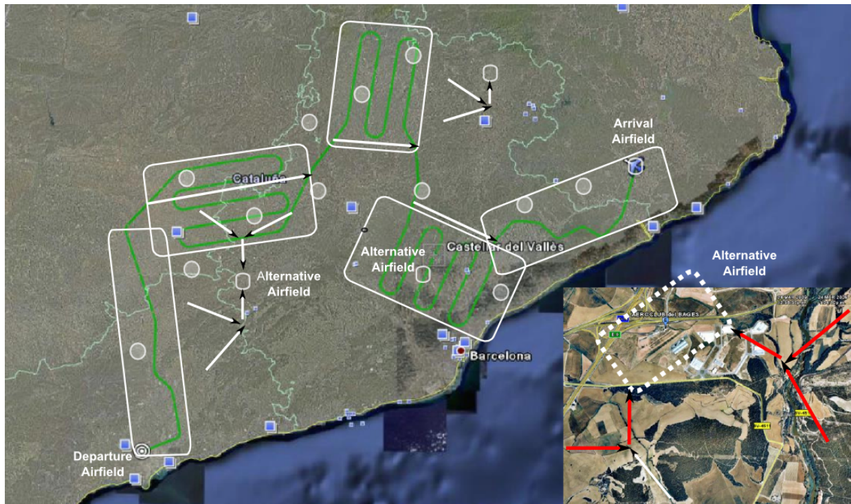
Figure 8. Example of flight dispatching with alternative airfields and emergency landing areas indicated.
