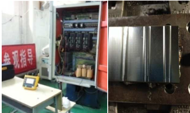
Fig.3 A power meter is used to measure power consumption (a), and end product of experiments carried out on a piece of 45 steel in dry machining(b).
