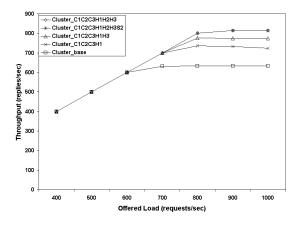
**Figure 11.** Throughput for a simple web server on a cluster-based TCP Server using HTTP/1.0
