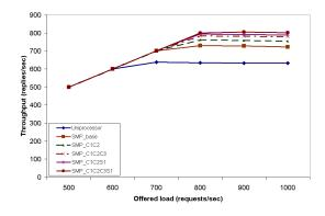
**Figure 9.** Throughput for a simple web server on a 2-Way SMP system using HTTP/1.0.
