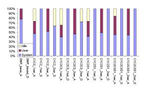
**Figure 8.** CPU usage at saturation for Apache on a 4-Way SMP Server. The suffix A denotes application processors and D denotes dedicated processors. The times are averaged over the entire set of processors.
