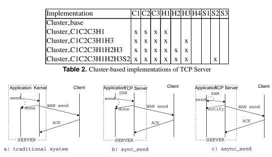
Figure 6. Comparison of the send operation in a traditional system with sync\_send and async send
