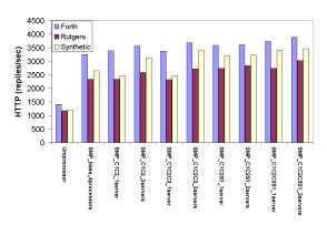
**Figure 7.** Throughput at saturation for Apache on a 4-Way SMP Server.
