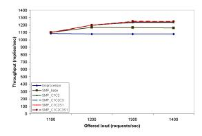
**Figure 10.** Throughput for a simple web server on a 2-Way SMP system using HTTP 1.1
