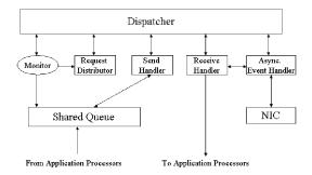
**Figure 4.** Organization of the TCP Server in an SMP-based server showing the different modules and their interaction with each other
