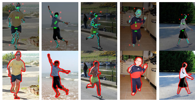
Fig. 4. Character segmentation results. The first row shows the automatically identified ‘definite human pixels’ (green) and ‘definite background pixels’ (red). The second row are results from graph-cut based segmentation.
