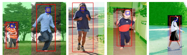
Fig. 2. Human detection results. The red frame is the bounding boxes of detected human. The blue frame indicates detected faces. The region overlaid in green contains 'definite background pixels'.
