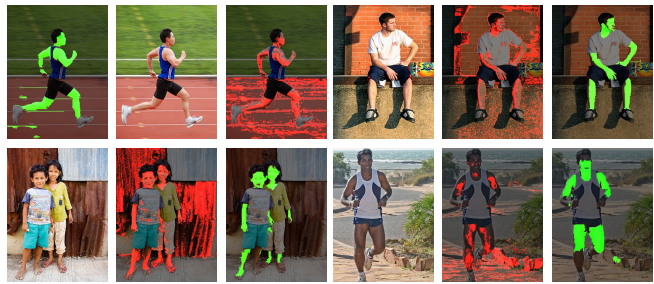
Fig. 3. Skin detection results. For each example, from left to right, they are the original image, detected skin pixels (red) according to [Jones and Rehg 2002], detected skin pixels (green) according to our method.
