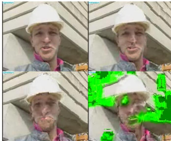
**Figure 2: Effect of transmission errors to a compressed video stream using the H.263 standard for a selected frame. Upper left: no transmission errors were present and the picture quality is as high as the bitrate allows; Upper right: 3% packet loss; lower left: 5% packet loss; lower right: 10% packet loss.**
