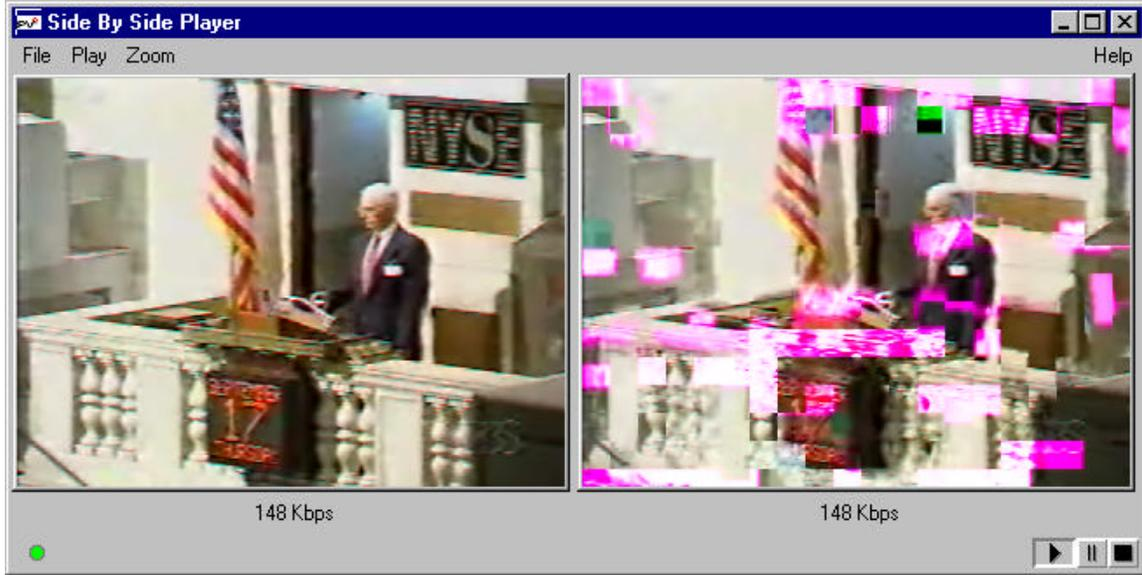
**Figure 9: A Comparison of Reconstructed Video Quality with and without Syntax Based Repair (Left: With syntax based repair, Right: Without syntax based repair. Identical bitstreams and error detection and concealment were used in both cases).**
