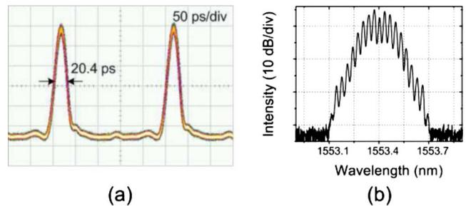
Fig. 4. (Color online) (a) Waveform and (b) optical spectrum of the experimentally generated optical pulses at 4 GHz.
