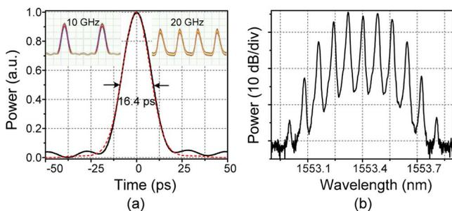
Fig. 3. (Color online) (a) Waveform and (b) optical spectrum of the experimentally generated optical pulses at 10 GHz.
