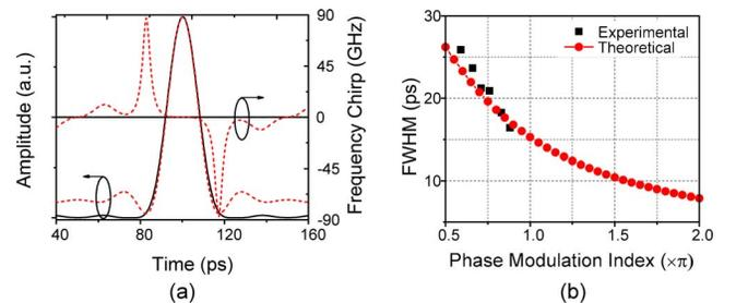
Fig. 2. (Color online) Theoretical study of the proposed pulse generator. (a) Comparison between the proposed method (solid curve) and pulse generation using a phase modulator and a dispersive element (dashed curve). (b) Dependence of the pulse FWHM on the phase-modulation index of the PolM.
