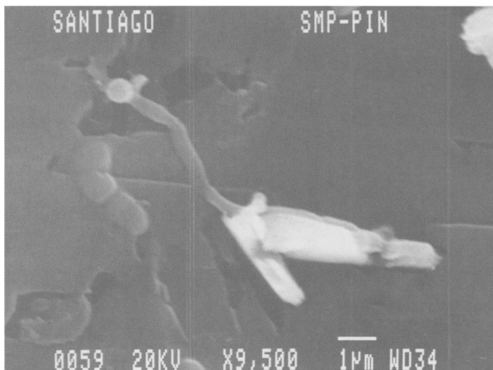
Fig. 8. SEM micrograph view of the exposed surface showing authigenic gypsum crystals nucleating on lichen hyphae on etched albite surface. Monasterio de S. Pinario, Santiago de Compostela, Spain.
