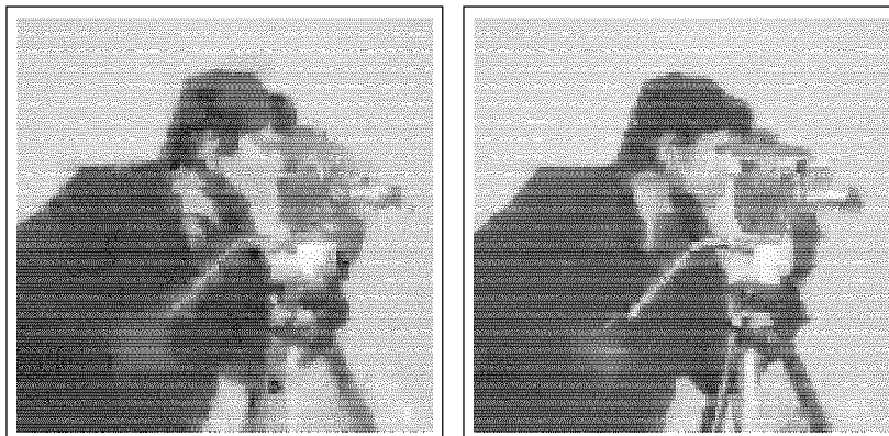
Figure 22. Detail of Cameraman at 30:1. (a) left: IIC4a, rmse = 21.61 . (b) right: IIC4b, rmse = 15.33 .
