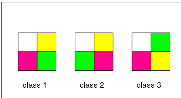
Figure 15. The three canonical orientations of a range or domain block. A block not in one of these forms can be so oriented by applying one of the eight isometric operations. The colors indicate a relative ranking of mean values of each quadrant.
