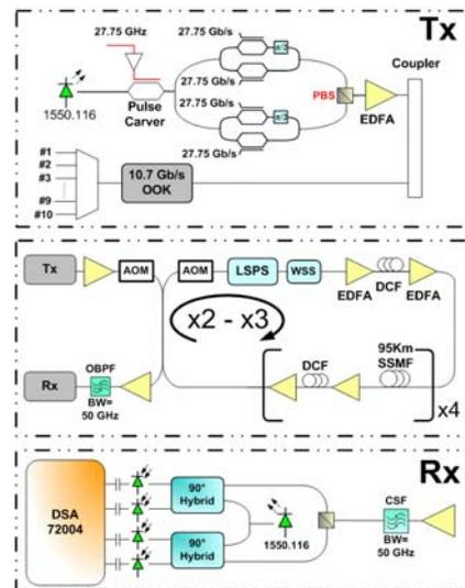
Fig. 1: System setup, WSS: wavelength selective switch, LSPS: loop synchronized polarization scrambler
