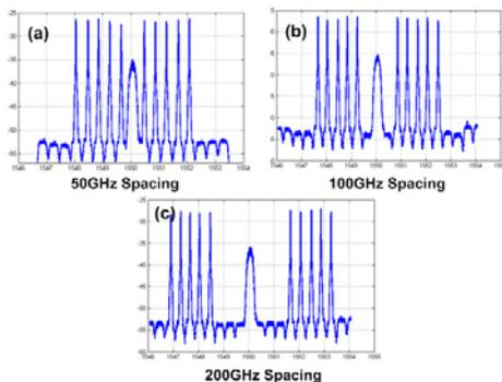
Fig. 2: Optical spectra of the 111-Gb/s signal with 10.7-Gb/s OOK signals at different channel spacing.
