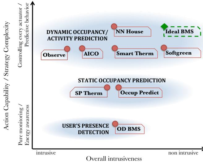
Fig. 9. Comparison of different BMS exploiting the “occupancy detection” intelligent functionality. The assessed BMS are: NNHouse [Mozer 1998], Observe [Erickson et al. 2011], AICO [Lu and Fu 2009], Smart Therm [Lu et al. 2010], Softgreen [Thanayankizil et al. 2012], SP Therm [Gao and Whitehouse 2009], Occup Predict [Vazquez and Kastner 2011], OD BMS [Agarwal et al. 2010].
