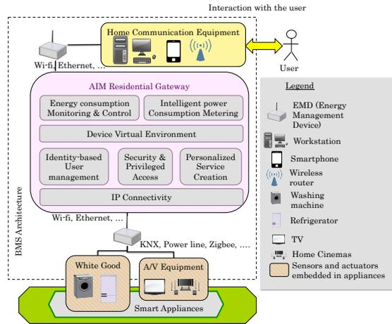
Fig. 4. AIM Reference Architecture.
