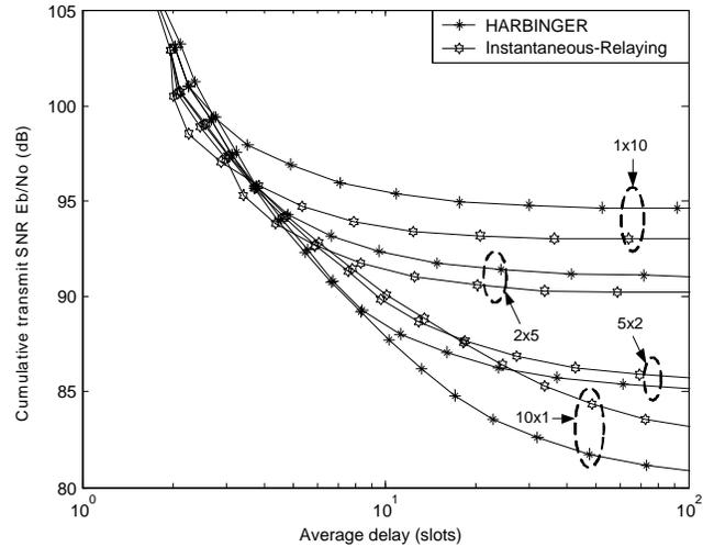
Fig. 4. The minimum cumulative transmit SNR required as a function of average delay for a  $u \times v$  line network comprising  $u$  equally spaced groups of  $v$  relays each.
