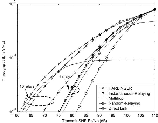
Fig. 1. The throughput of a line network as a function of the per-burst transmit SNR for  $K_r = \{1, 10\}$  equally spaced relays without a delay constraint. Results for direct transmission link ( $K_r = 0$ ) are also shown. All protocols use code-combining.
