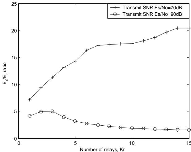
Fig. 5. The minimum required ratio of transmit vs. receiver energy dissipation per symbol for HARBINGER to outperform multihop in an equidistant line network with  $K_r$  relays.
