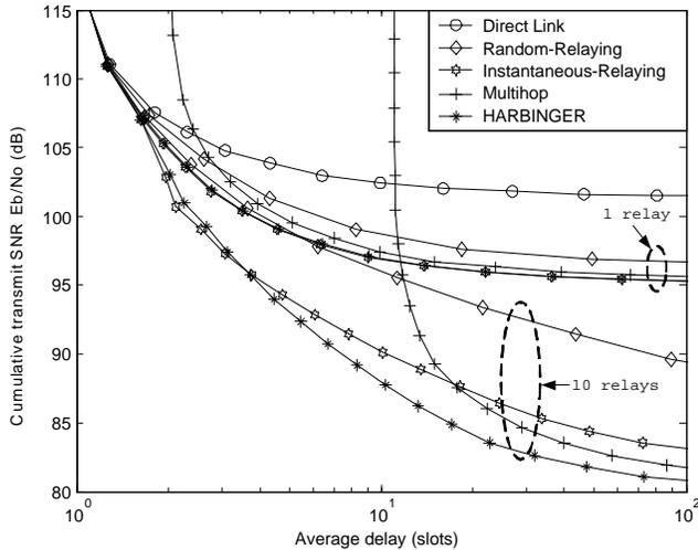
Fig. 3. The cumulative transmit SNR  $\mathcal{E}_b/N_o$  as a function of average delay in a line network with  $K_r = \{1, 10\}$  relays. Results for direct transmission link ( $K_r = 0$ ) are also shown.
