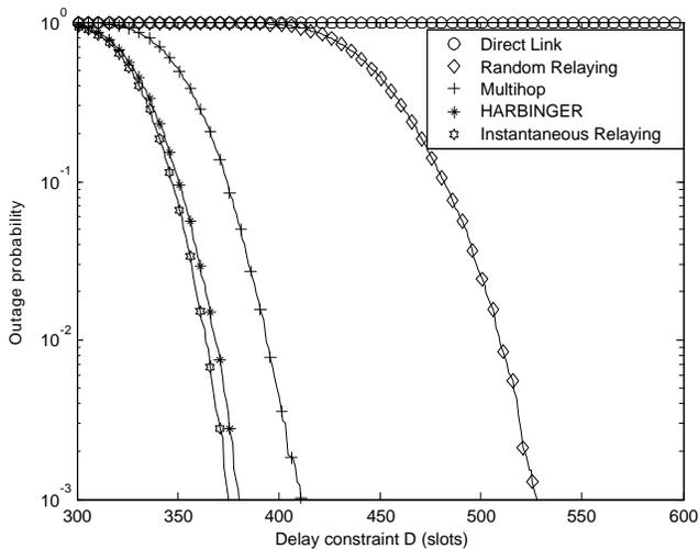
Fig. 8. The outage probability of different relaying protocols as a function of delay constraint for a single relay line network with transmit SNR  $\mathcal{E}_s/N_o = 70$  dB and code-combining. A threshold in the outage probability of direct link appears around  $D=1400$  (not shown).
