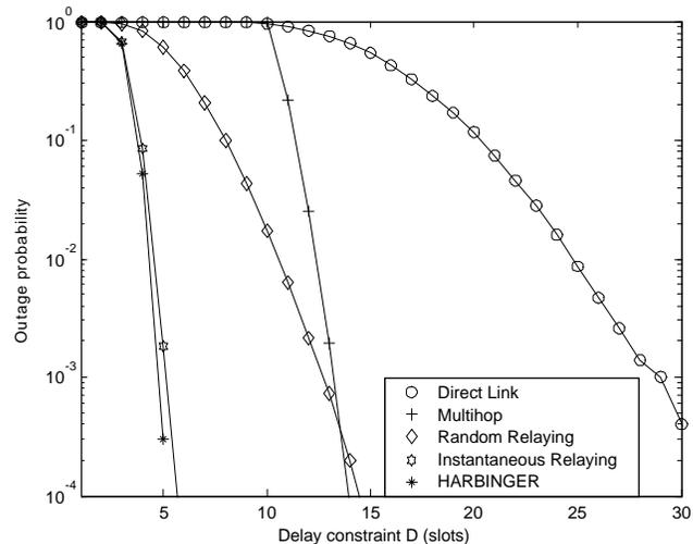
Fig. 11. The outage probability of different relaying protocols as a function of delay constraint for a 10 relay line network with transmit SNR  $\mathcal{E}_s/N_o = 90$  dB and code-combining.
