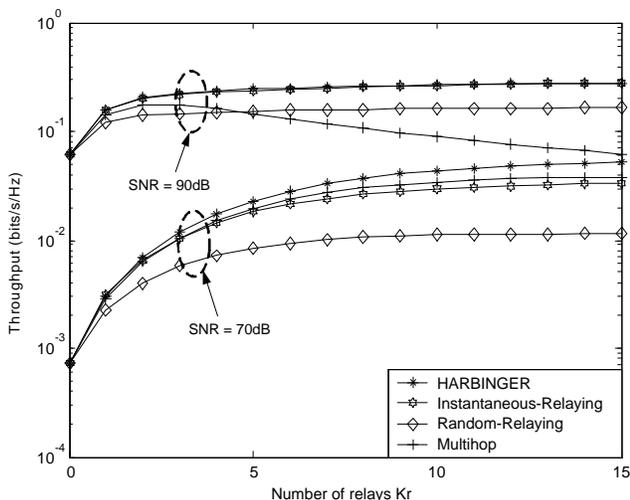
Fig. 2. The throughput of a line network as a function of the number of relays for two different per-burst transmit SNRs.
