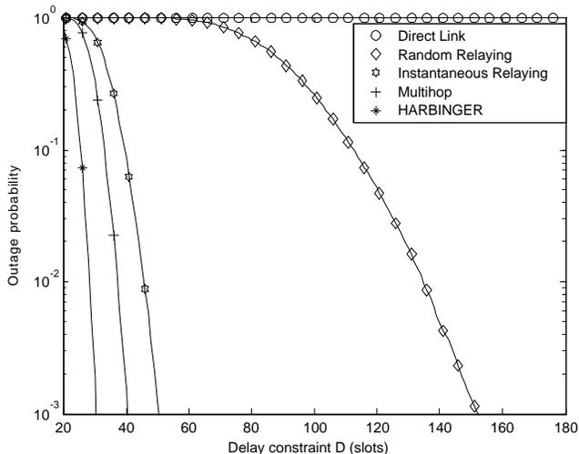
Fig. 9. The outage probability of different relaying protocols as a function of delay constraint for a 10 relay line network with transmit SNR  $\mathcal{E}_s/N_o = 70$  dB and code-combining.
