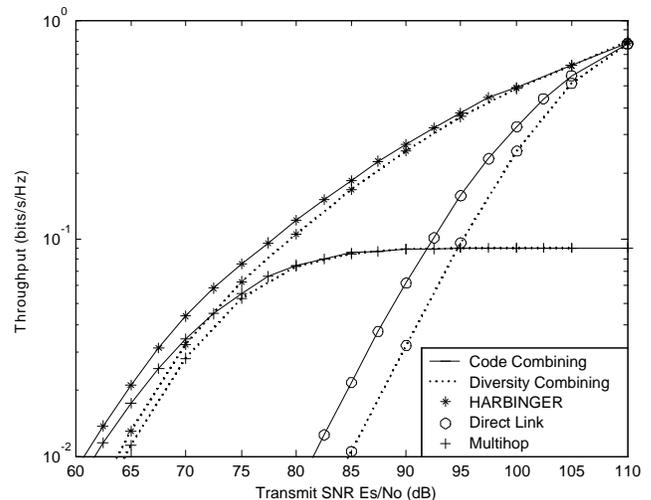
Fig. 6. The throughput of code- and diversity-combining in an equidistant line network with  $K_r = \{1, 10\}$  relays as a function of the per-burst transmit SNR.
