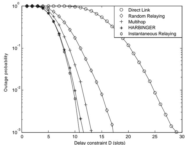
Fig. 10. The outage probability of different relaying protocols as a function of delay constraint for a single relay line network with transmit SNR  $\mathcal{E}_s/N_o = 90$  dB and code-combining.
