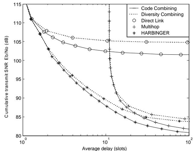
Fig. 7. The cumulative transmit SNR  $\mathcal{E}_b/N_o$  of code- and diversity-combining as a function of average delay in a line network with  $K_r = \{1, 10\}$  relays.
