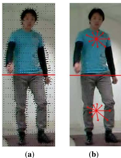
Figure 7. An example of histogram of oriented gradient (HOG) descriptor: (a) the image gradients of local grids; (b) the HOG descriptor with nine bins for the upper body and the lower body [59].
