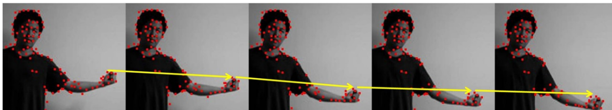
Figure 8. An example of fist tracking using one Lucas-Kanade-Tomasi (LKT) tracker. The red dots denote the LKT feature points, and the yellow line denotes the tracking by one LKT tracker [100,101].
