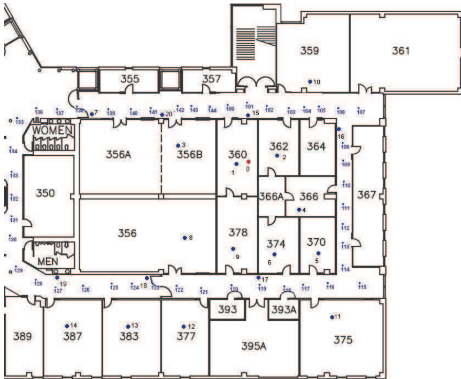
Fig. 4. Deployment of WSN-based Tracking System at the Peter Kiewit Institute (PKI)
