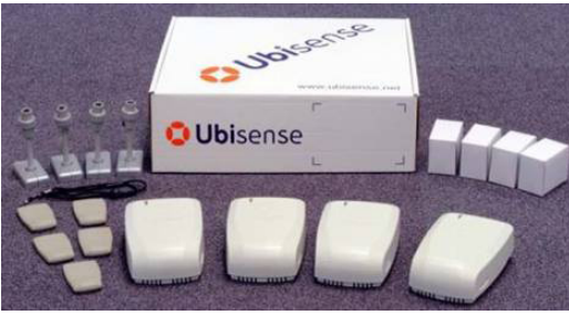
Fig. 15. Hardware of the Ubisense System in a Academic Research Package: five tags (left) and four sensors (right)
