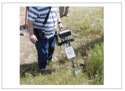
**Figure 2.** The light-weight analyzer for buried remains and decomposition odor recognition (LABORADOR) is an example of a chemical sensing device that was specifically designed for locating chemical scent plumes associated with human decomposition
