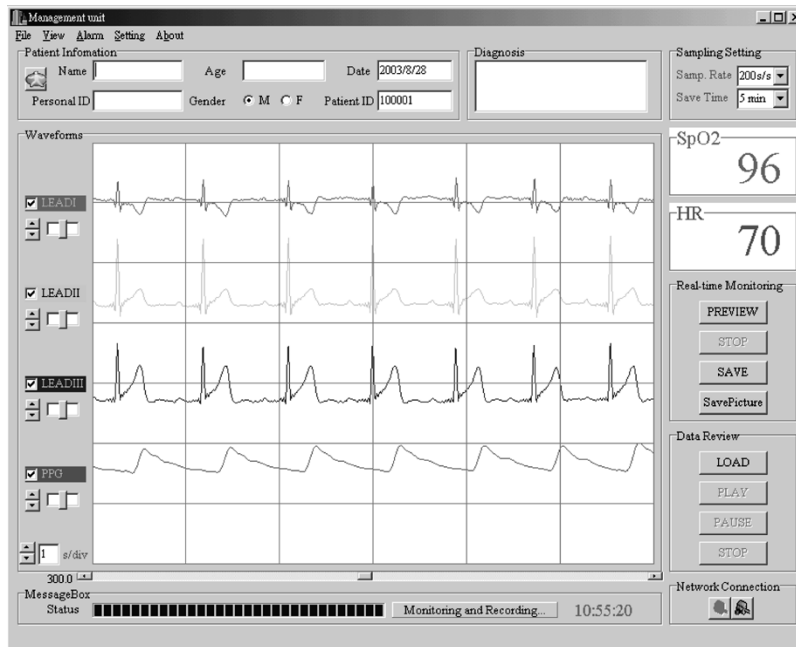
Fig. 8. Main control window and vital-sign signals display of the management unit.
