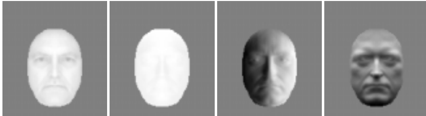
Fig. 1. The albedo and normals estimated directly assuming known light source directions and without using robust techniques to remove specularities and shadows. The leftmost image is the albedo, the next three images are the z , x , and y components of the surface normal respectively. Observe that the estimated albedo appears to get darker near the boundaries of the face causing the albedo image to appear to be non-flat. This is due to failure to treat the shadows correctly.
