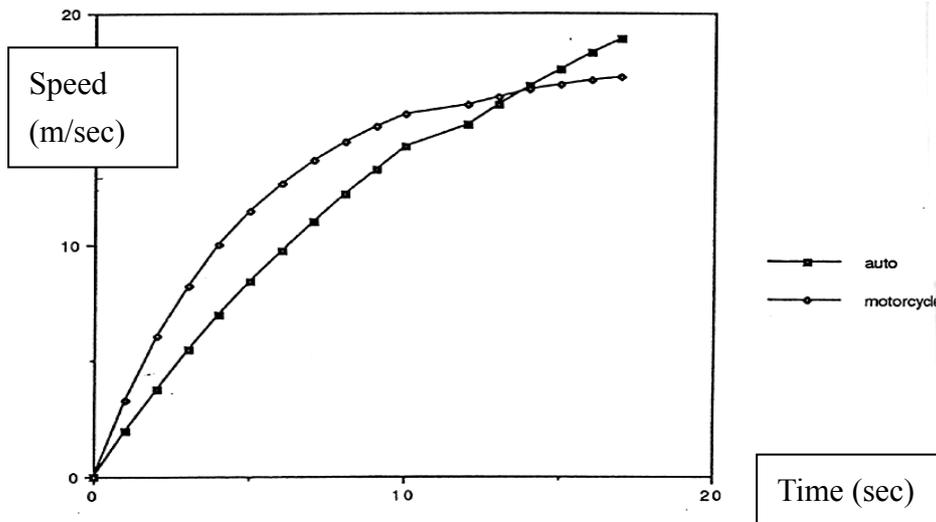
Figure 16: Cruise speed after starting of motorcycle and automobile
