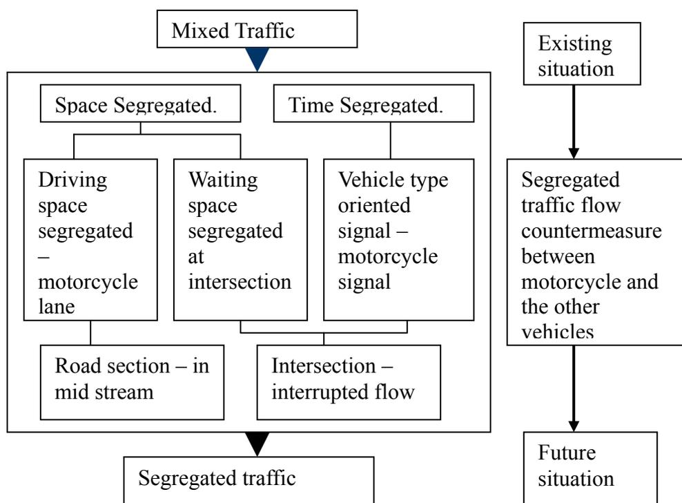
Figure 26: The concept structure from mixed traffic to segregated traffic (Hsu, 1997)
