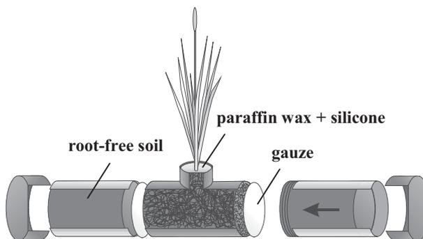
**Figure 1:** Experimental air-tight vessels divided by gauze into three parts: a central part containing rooted soil and two lateral parts with root-free soil separated by gauze with a clear mesh of 30  $\mu\text{m}$ . The arrow indicates the treatment of the two lateral soil columns, which were separated from the central part, frozen, pushed out (arrow) of the vessel, and cut into 2 mm slices.
