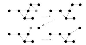
Fig. 5. Repeatedly removing *chains* and *parallel pipes* from a water network graph. Chains (nodes with two edges) and parallel pipes (parallel edges) are marked gray
