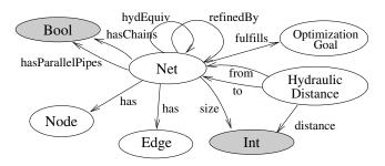
Fig. 3. Simplified version of a water supply network domain ontology
