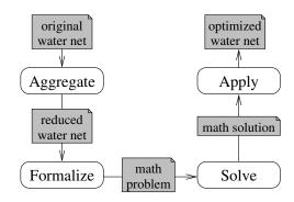
Fig. 2. Abstract workflow of optimizing water supply networks
