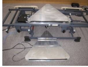
Fig. 2 Two specially designed force plates placed at the positions of the feet and hip of subjects
