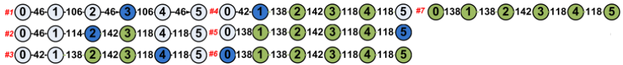
Fig. 5 Hierarchical re-indexing of 6-Module climber configuration graph. Module 3, the master starts VVMP and freezes its edges, the process is continued by 2, 4, 1, 5, and 0.
