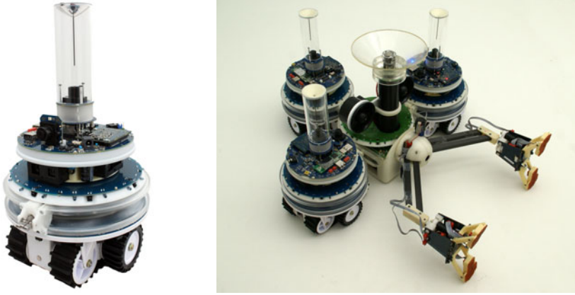
Fig. 4 Left: Foot-bot robot. Right: Possible positioning of foot-bot robots around the hand-bot to provide movement on the ground.
