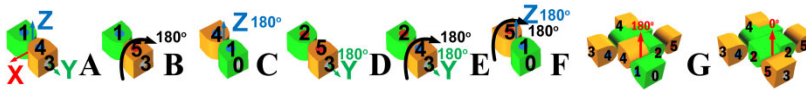
Fig. 3 (A)-(F) Examples of SuperBots with identical 3D shapes. In B, E and, F, the middle servo rotates 180° (G) Two isomorphic configurations with a module rotated around a symmetry line.
