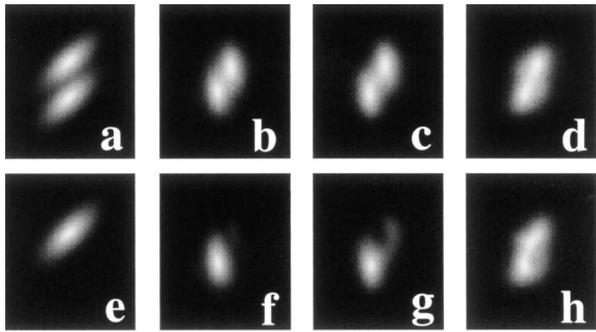
Fig. 2. Gray-scale images of (a–d) the total intensity distribution and (e–h) the intensity distribution of a single elliptic soliton beam at (a, e)  $z = 0$  cm, (b, f)  $z = 1.6$  cm, (c, g)  $z = 2.12$  cm, and (d, h)  $z = 4.7$  cm.
