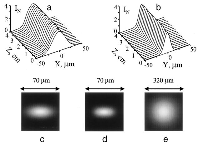
Fig. 1. Intensity evolution of an elliptic Gaussian soliton beam when  $r = 3$ ,  $\theta_{0x} = 0.283^\circ$ ,  $\theta_{0y} = 0.2^\circ$ , and  $\Delta n = 1.42 \times 10^{-4}$ : a, along the  $x$  axis; b, along the  $y$  axis. Gray-scale images: c, input and d, output elliptic soliton and e, its diffraction after 2 cm.
