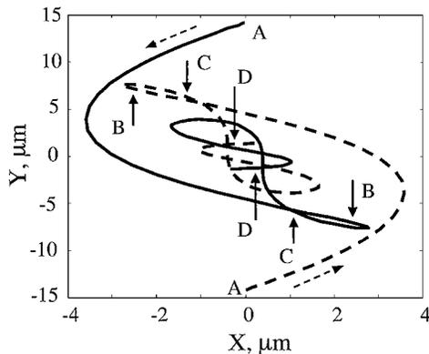
Fig. 3. Trajectories of the centers of gravity in the transverse plane of two elliptic soliton beams initially centered on the  $y$  axis and tilted at  $45^\circ$  with respect to  $x$  axis. Points A, B, C, and D occur at  $z$  values of 0, 1.6, 2.12, and 4.7 cm, respectively.
