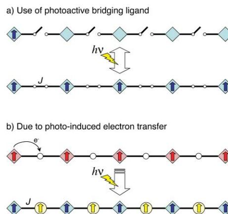
Fig. 7 Proposed design of photo-induced SMM-network compounds.
