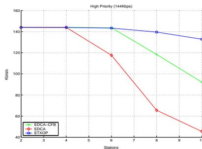
Figure 5. AC3's flow (144kbps) data rate
