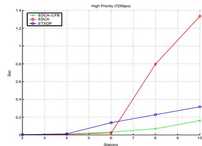
Figure 8. AC3's flow (72kbps) packet delays
