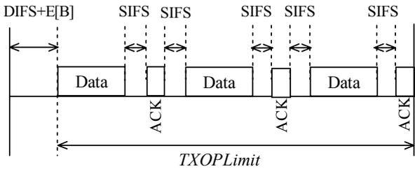
Figure 1. Medium access when enabling TXOPlimit
