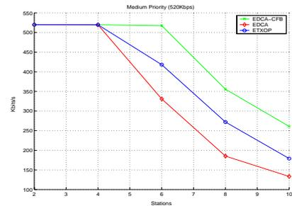
Figure 6. AC2's flow (520kbps) data rate
