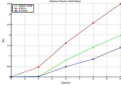
Figure 11. AC2's flow (1040kbps) packet delays
