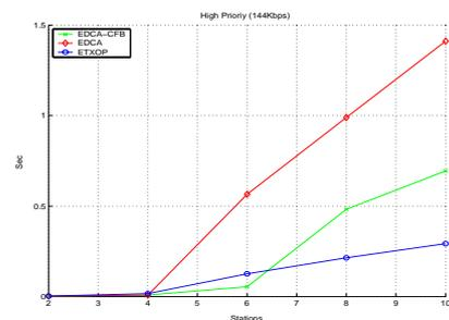
Figure 9. AC3's flow (144kbps) packet delays
