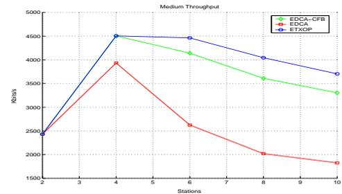
**Figure 3. Overall network throughput**
