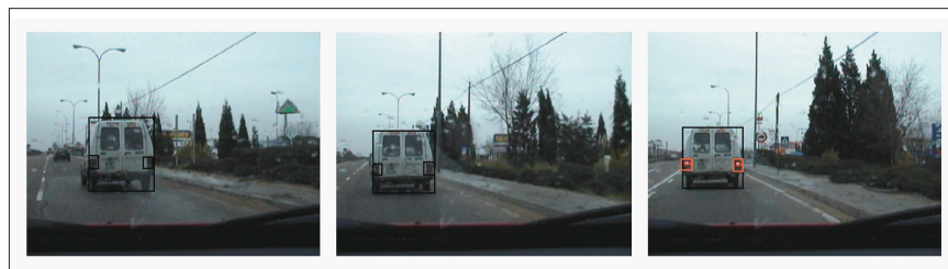
Figure 10. Sudden-braking detection. Once the system locates the brake lights, it continuously monitors their luminance to detect brake-light activation.
