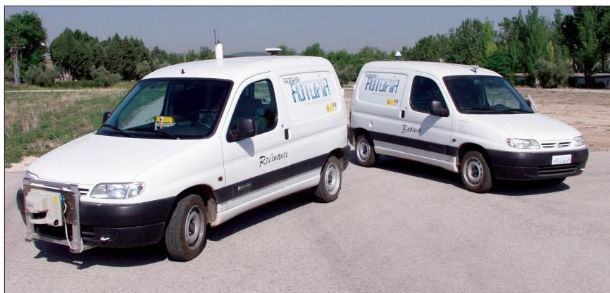
Figure 1. The AUTOPIA testbed vehicles. An embedded fuzzy-logic-based control system controls both speed and steering in each Citroën Berlingo.
