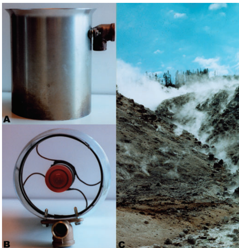
Fig. 1. Fumarole collection images. A. Portable steam collector, side view; height = 15 cm, diameter = 10 cm. B. Top view with cover off showing placement of orange-capped sterile 50 ml conical polypropylene tubes. C. Photo of Roaring Mountain site showing example fumarole steam vents alongside the spring water channel.
