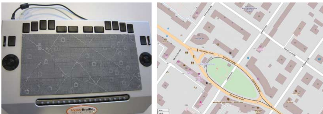
Figure 3. A part of Dresden City map presented by the HBMap system (left: non-visual representation on a HyperBraille display; right: a screenshot of the vision-based map from the OSM site). (The map rendered is around the area of 'Nürnberg Street' in the city of Dresden.)
