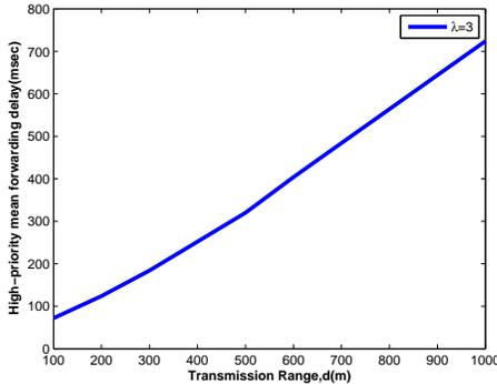
Fig. 4. Average delay of high-priority message dissemination for H = 5 hops of communication as functions of the transmission range
