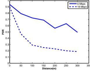
Fig. 3. PDR vs. separation distance under different data rates in the Rural Road(RR) environment (with 95% Confidence Interval). Here, data rate is 6 Mbps and 18 Mbps. Transmission power is 20 dBm.
