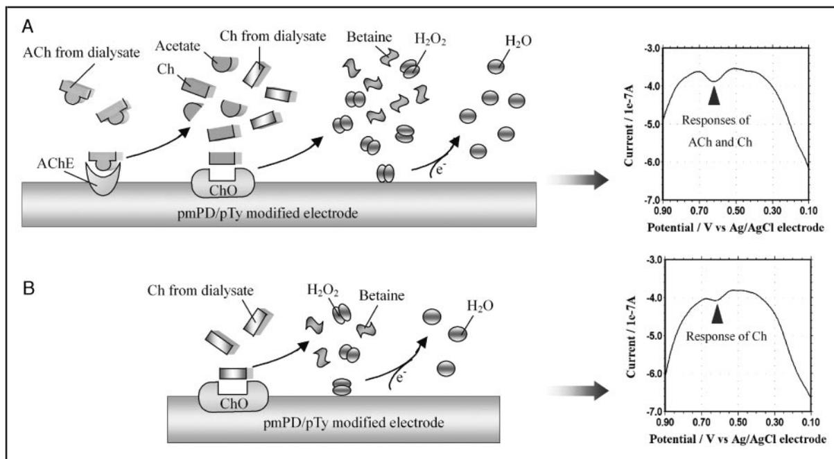
**Fig. 2.** Schematic diagram of sensors for the measurement of ACh.
