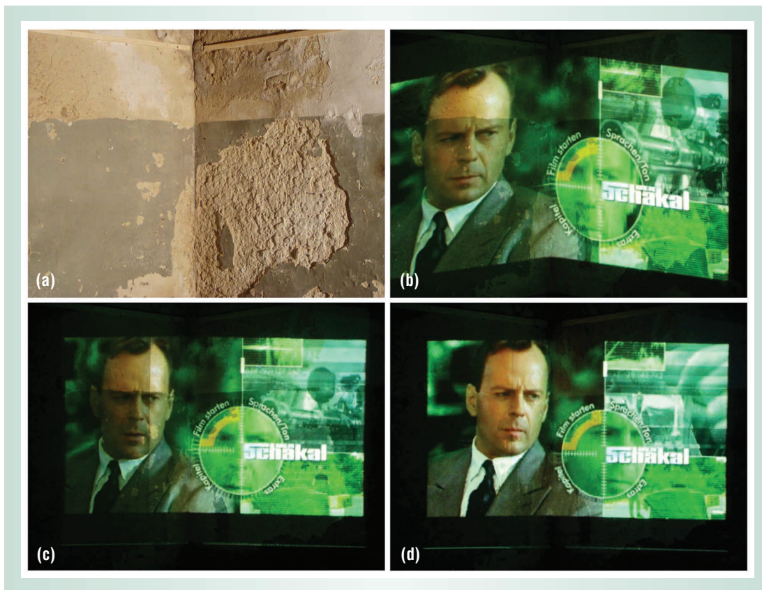
Figure 2. Projecting images onto environmental surfaces. (a) A scruffy corner serves as the projection surface. (b) The uncorrected image. (c) The projector system corrects the image's geometry and, finally, (d) its color. Displayed content: The Jackal, Universal Pictures.
