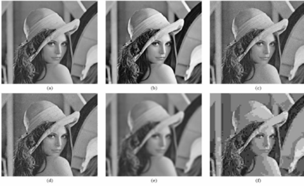
Figure 4. (a) Original Image ‘‘Lena’’ 512 x 512. (b) Contrast-stretched Image, MSE = 225, SIM = 0.9327. (c) Gaussian Noise Image, MSE = 225, SSIM = 0.3891 (d) Impulsive Noise Image, MSE = 225, SSIM = 0.6494 (e) Blurred Image, MSE = 225, SSIM = 0.3461 (f) JPEG Image, MSE = 225, SSIM = 0.2871
