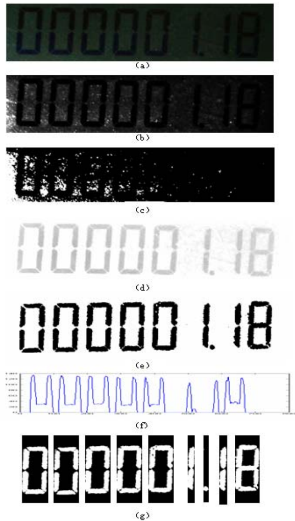
Figure 4. The test image and the results of each step of the preprocessing
