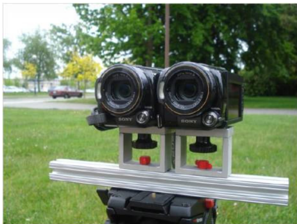
Figure 1. Stereo camera setup consisting of two identical HD camcorders.
