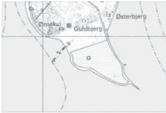
Fig. 5.12: The Nekselø site. Dots mark the positions of in situ wooden poles from Stone Age fish weirs. Lines of poles have been found over a distance of c. 250 m and air photographs show dark shadows in continuation of the presently recorded constructions indicating that they stretch much further out into the sea. The weirs have been re-built many times over a period spanning from the Late Mesolithic and into the Middle Neolithic. A settlement, representing the very same periods of use, has been excavated close to the landward end of the constructions (the Ørnekul site, marked with a filled in square) (Graphic by T. Eriksen, The National Cultural Heritage Agency of Denmark).
