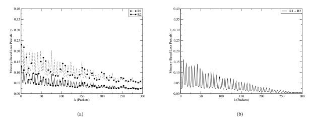
Fig. 7. Experiment 2: Distance: Memory-based loss correlation (10 Feet, 16 Mb/s) of  $R_1$  and  $R_2$  (a) separately (b) together.
