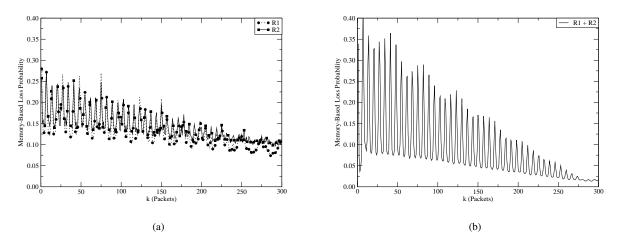
Fig. 8. Experiment 2: Distance: Memory-based loss correlation (40 Feet, 16 Mb/s) of  $R_1$  and  $R_2$  (a) separately (b) together.
