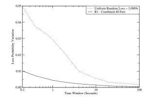
Fig. 10. Experiment 2: Distance: modified Allen Deviation (40 Feet, 16 Mb/s) of  $R_1 + R_2$ .
