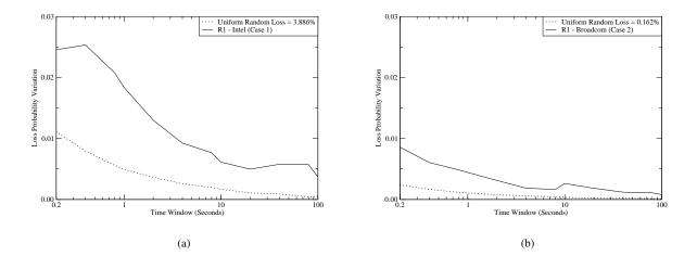
Fig. 4. Experiment 1: Allen Deviation of (a) Case 1 Node  $R_1$  (b) Case 2 Node  $R_1$ .
