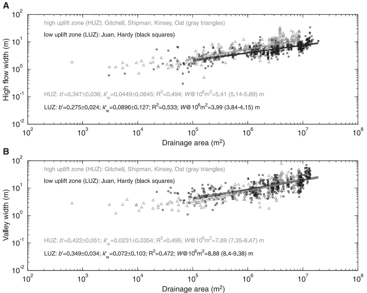
Fig. 4. Graphs of width vs. drainage area for (A) high-flow width and (B) valley width. High uplift zone data are gray triangles, low uplift zone data are black squares. Lines are least-squares best-fit power-law regressions (heavy lines), with associated 95% confidence hyperbolae (fine lines), for the two datasets, with  $A > 10^5 \text{ m}^2$  (Hamilton, 1992). See Table 3 for data for individual streams.
