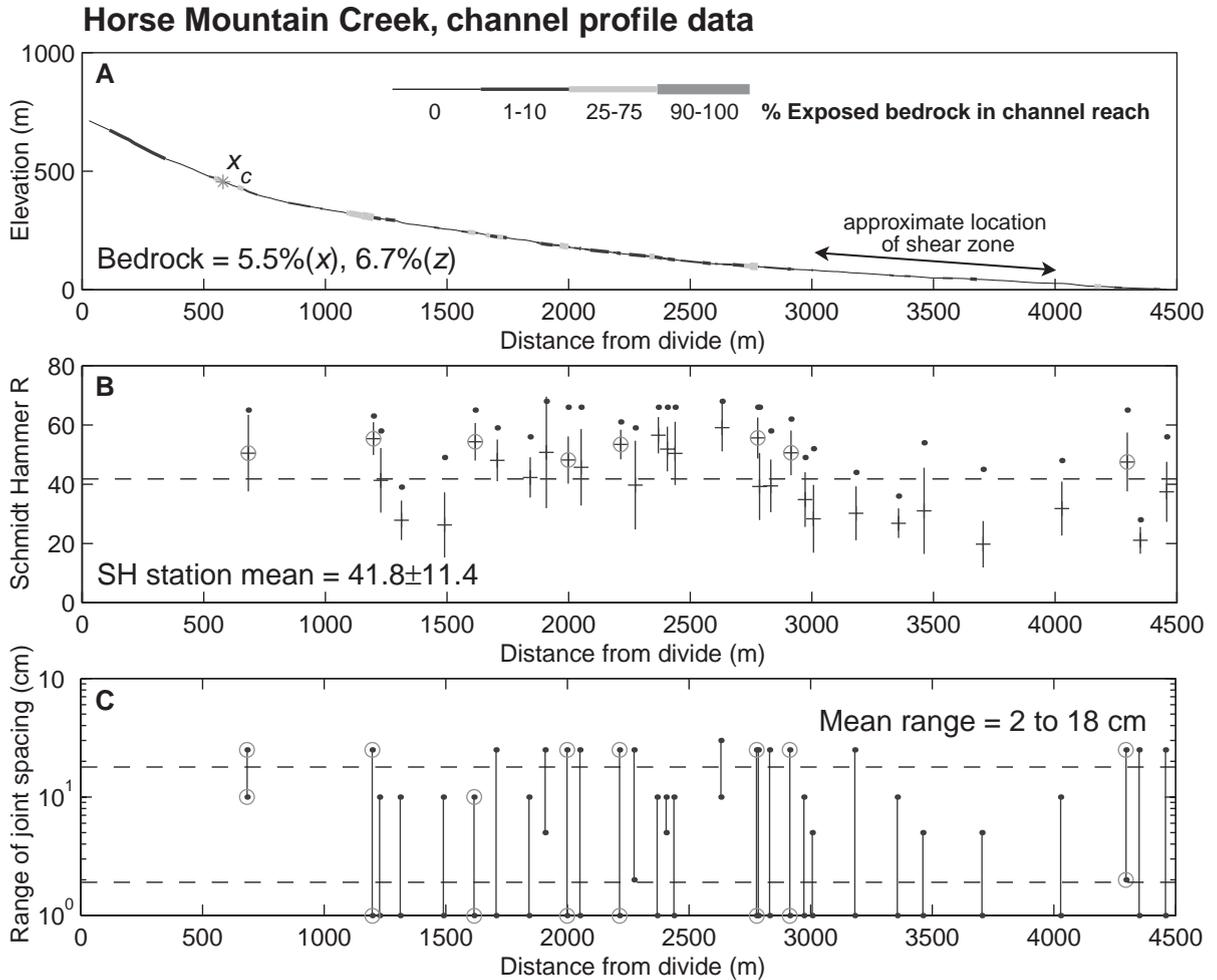
Fig. 10. Channel profile data for Horse Mountain Creek in the intermediate uplift zone. See Fig. 8 for description. (A) Arrow indicates the section of the channel oriented along a major shear zone.
