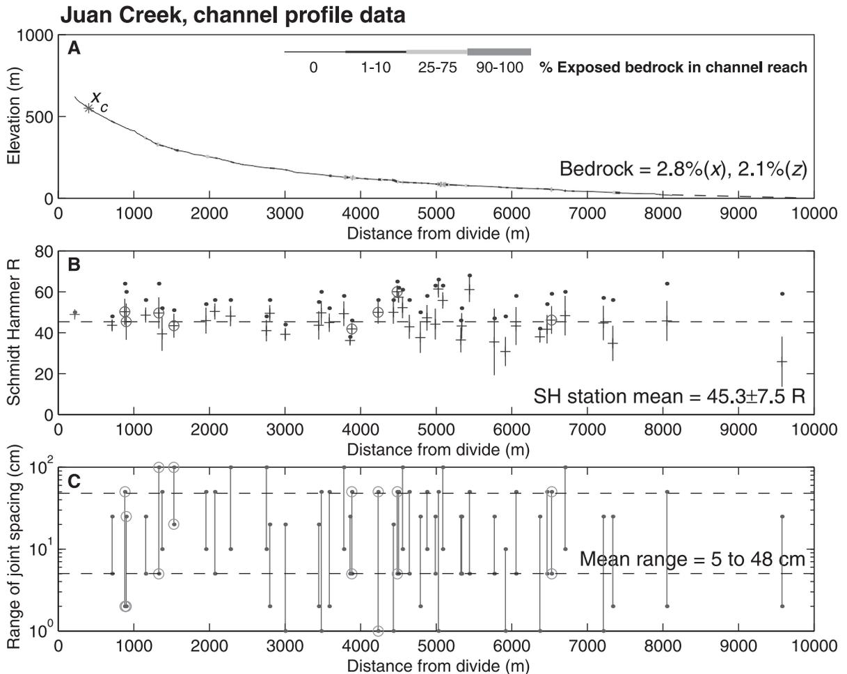
Fig. 9. Channel profile data for Juan Creek, in the low uplift zone. See Fig. 8 for description. (A) Area not included in the field survey marked by dashed line.
