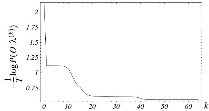
Figure 6-14: The Baum-Welch algorithm can stall over several iterations, until further improvements are realized.
