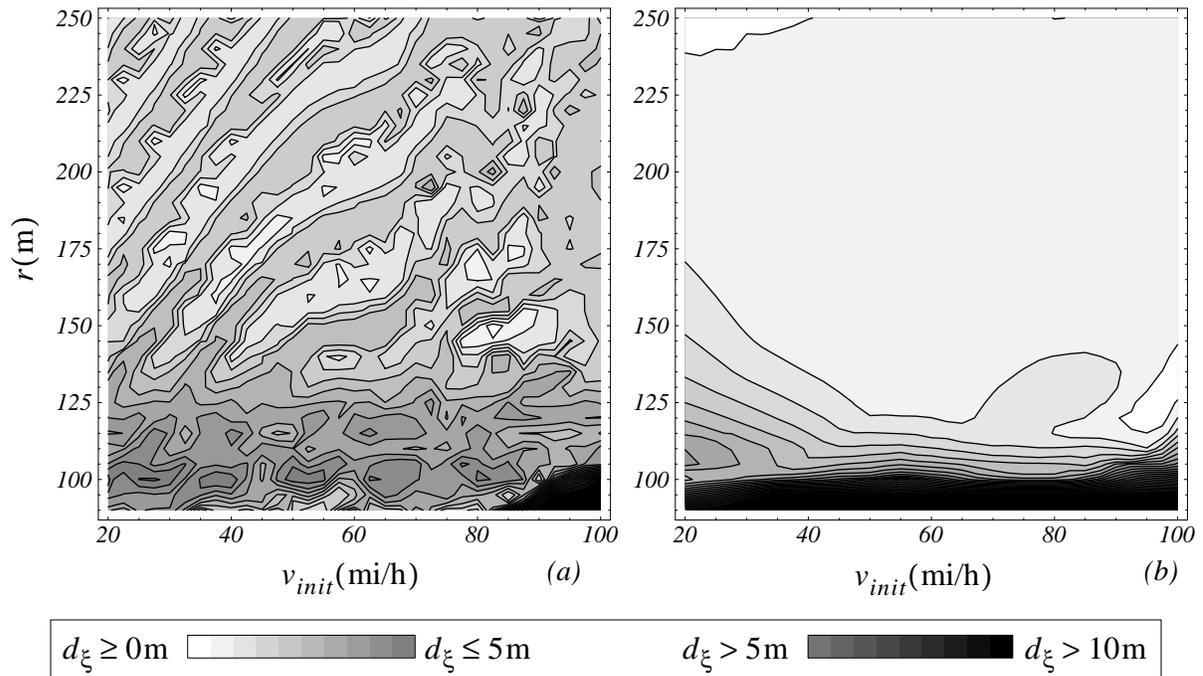
Figure 4-14: Groucho's stability profiles through the s-curve for (a) the  $Cq$  model and (b) the  $Ck$  model (lighter colors are better).
