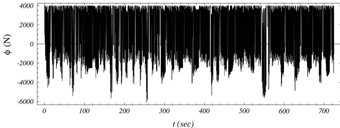
**Figure 4-10: Larry's  $Ck$  model control with one hidden unit added. Note that the additional hidden unit causes significant (not really beneficial) high-frequency noise.**
