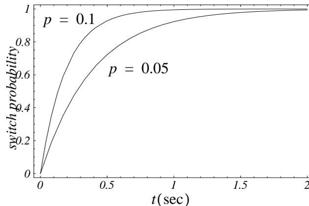
**Figure 5-12: Probability of a switch after  $t$  seconds (at 50 Hz) when the probability of a switch at each time step is  $p$ .**
