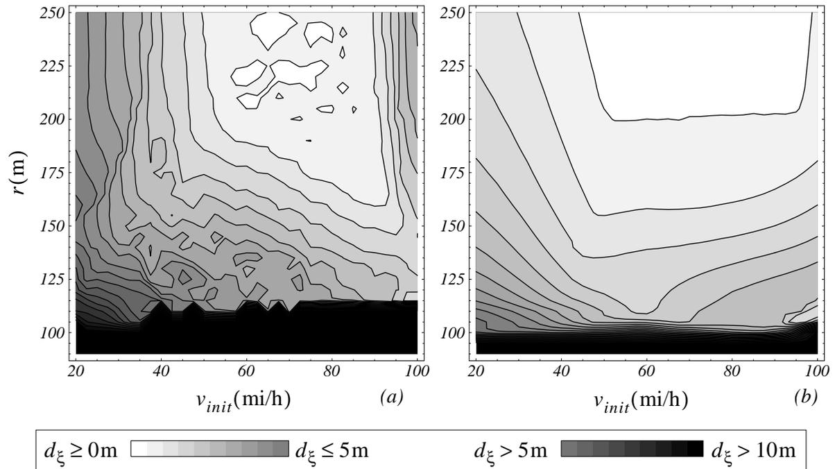
Figure 4-12: Larry's stability profiles through the s-curve for (a) the  $Cq$  model and (b) the  $Ck$  model (lighter colors are better).
