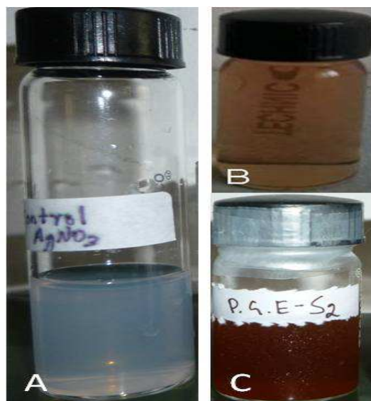
Figure 1. Colour changing during synthesis of AgNPs. A) 1mM AgNO 3 B) Pomegranate Peel extract C) AgNPs after 24h incubation in room temperature (Reaction Mixture)
