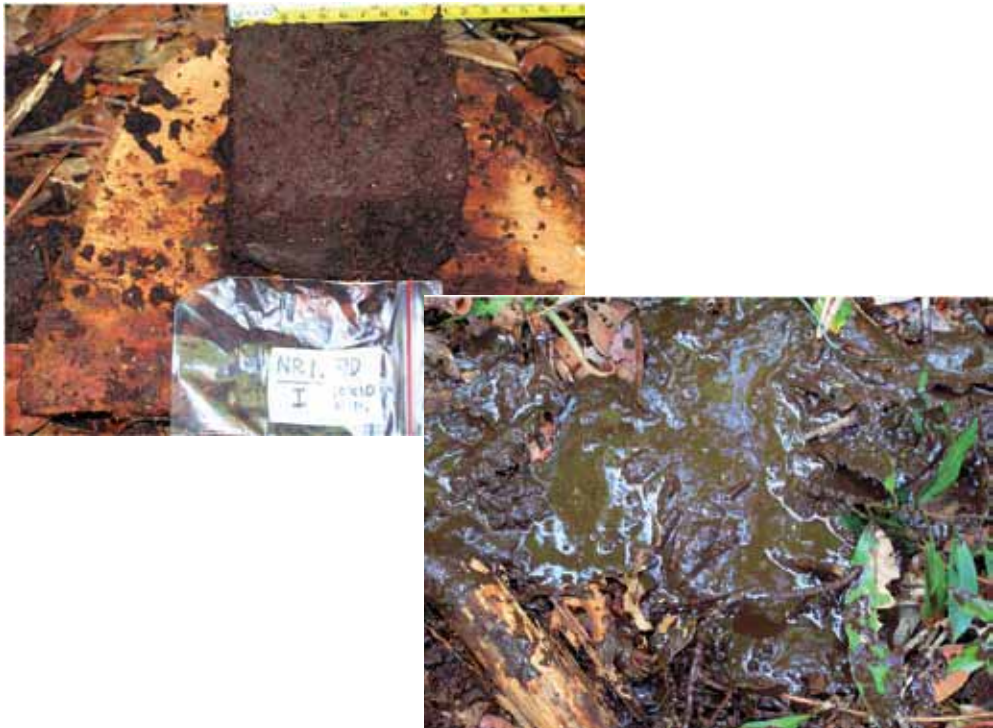
Figure 12. Cubical and fluid peat samples Cubical (left) and fluid (right) samples taken with an Eldeman auger from depths below the watertable
