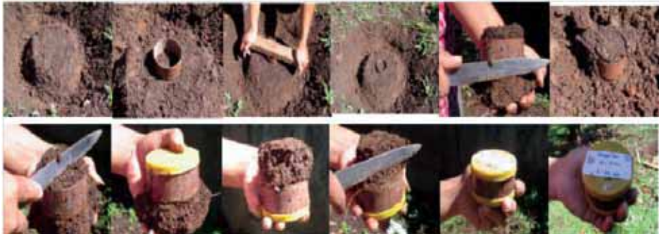
Figure 11. Stages of undisturbed soil sampling using soil core (From top left to bottom right)
