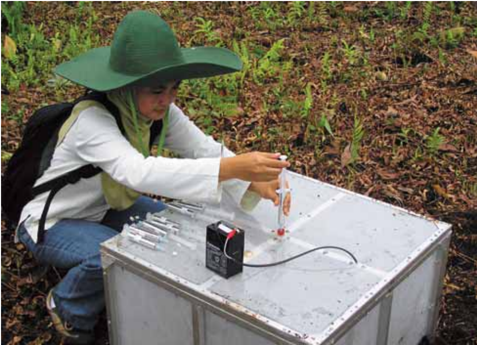
Figure 19. Gas sampling from a closed chamber for gas concentration measurement using gas chromatography
