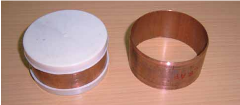
Figure 10. Soil core (soil ring) for undisturbed soil sampling Soil rings with and without caps. Ring diameters typically range 5–7.5 cm and heights 2.5–6 cm. Rings of small diameter may cause more damage to soil samples.
