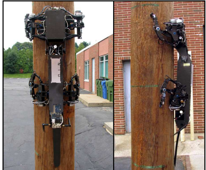
Fig. 1: Dorsal and lateral views of the RiSE Version 3 climbing robot. Four powerful legs, each with two actuators, grip a wooden telephone pole using claw-like appendages.
