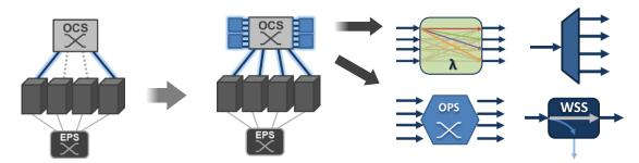
Fig. 1. A variety of optical functionalities can be used to enhance the optically connected data center network, increasing bandwidth granularity and connectivity, and yielding more efficient utilization of the photonic layer.
