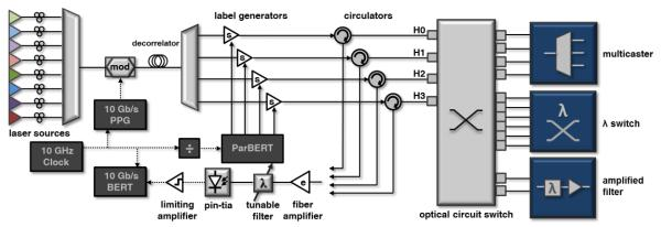
Fig. 2. The experimental setup emulating four nodes transmitting at up to 80 Gb/s utilizing a reconfigurable set of optical network functions.
