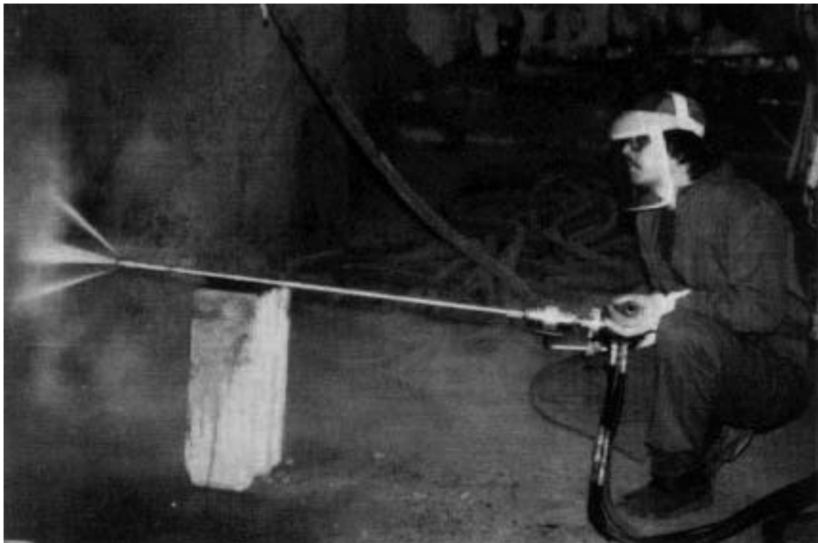
Figure 8. 40,000 psig handheld rotary drill provided by Jarvis Clark Co.
