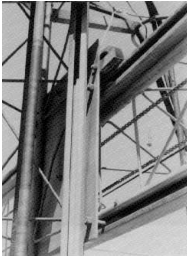
Figure 5. Main platform view with horizontal bar, high pressure pipe and feed screw.
