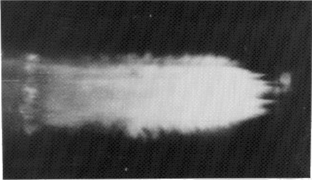
Plate 1 Waterjet in flight (TEST 7) showing "fingers" and droplet shroud at front of jet
