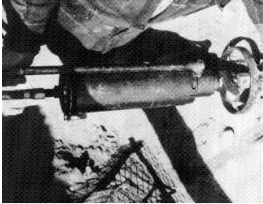
Figure 2. Rotary cleaning head with sizing ring used in Phase II.
