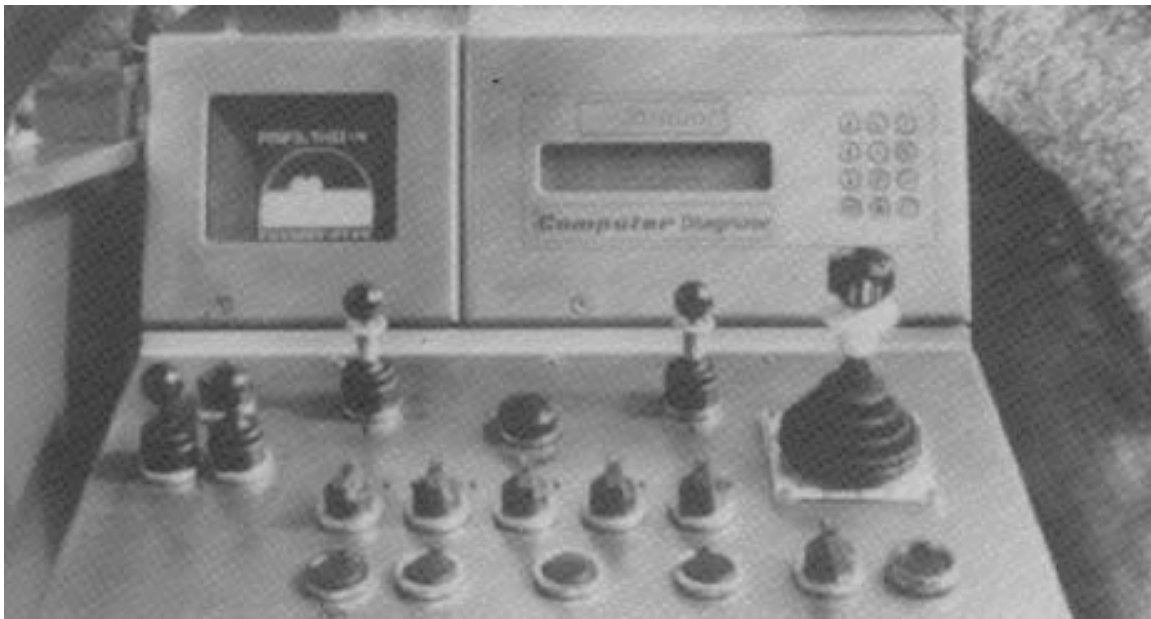
Fig. 13 The mining machine of the future: Computer-controlled alignment and profile control, machine health monitoring and diagnostic system of Eickhoff, Germany.
