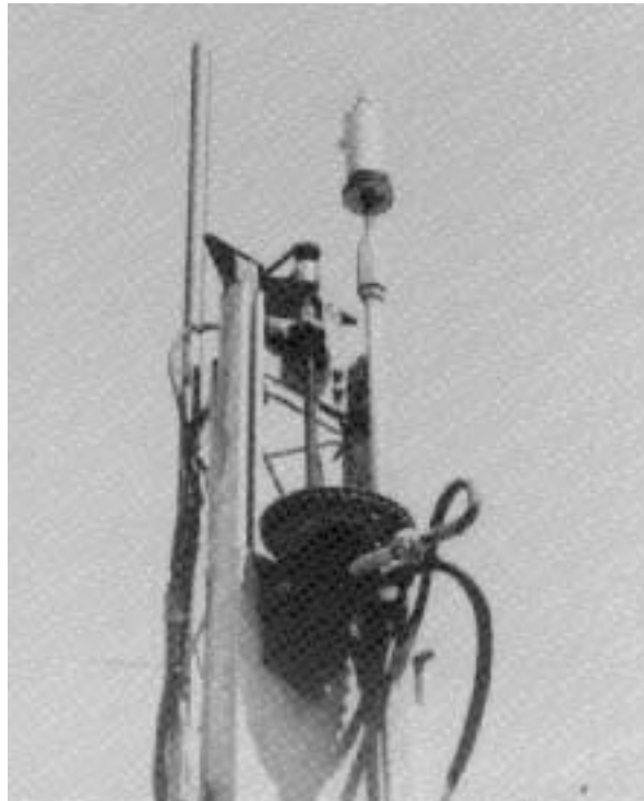
Figure 3. Lance feeding device and lance running gear. Rotary coupling on the top of high pressure pipe.
