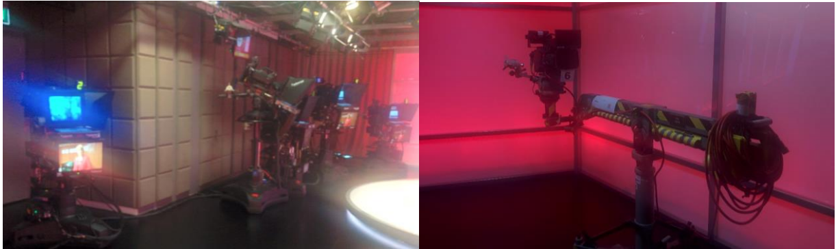
Figure 3: A series of (standard) studio cameras (left) and a jib-arm camera (right).
