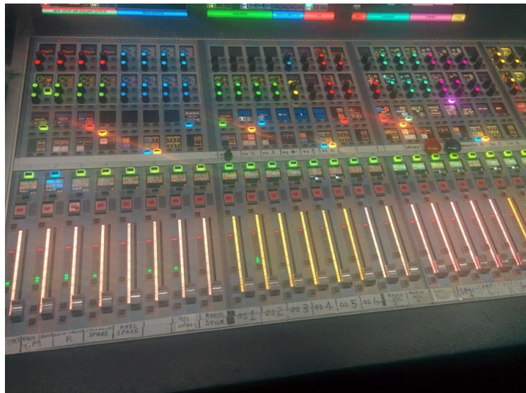
Figure 4. Sound mixing desk. The sliders that alter the volume for each microphone are found at the bottom of the mixer.
