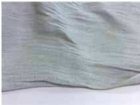
Fig. 28. Weaved fabric (0/ 90) with twisted yarns
