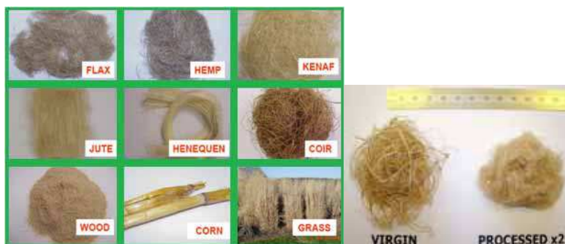
Fig. 4. (a) Some natural fibre, (b) Unprocessed and Processed hemp fibres (source: University of Exeter)
