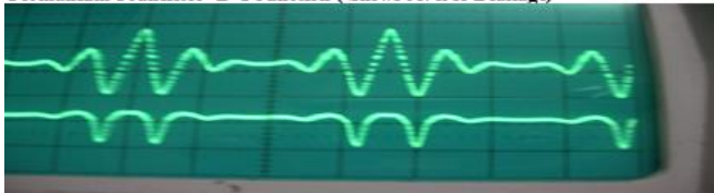
Fig. Germanium Transistor B-C Junction (Shows reverse Leakage)
