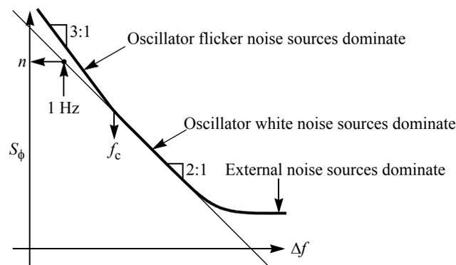
$S_\phi$  is not directly observable and often difficult to find. So instead oscillator phase noise is often characterized using  $L$ , the spot noise power of the output voltage  $S_v$ , normalized
