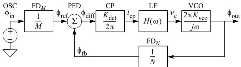
The derivation of the model begins with the identification of those signals that are best represented by their phase. Many blocks have large repetitive input signals with their outputs being primarily sensitive to the phase of their inputs. It is the signals that drive these blocks that are represented as phase. They are identified using a  $\phi$  variable in Figure 2. Notice that this includes all signals except those at the inputs of the LF and VCO.
