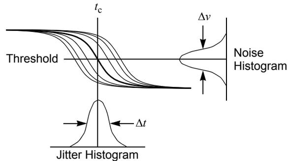
Generally  $n_v$  is not stationary, but cyclostationary (refer back to Section 6.1). It is only important to know when the noisy periodic signal  $v_n(t)$  crosses the threshold, so the statistics of  $n_v$  are only significant at the time when  $v_n(t)$  crosses the threshold,
