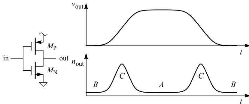
produced by the circuit is periodically sampled to create a discrete-time random sequence, as shown in Figure 9. SpectreRF then computes the power-spectral density of the sequence. The sample time should be adjusted to coincide with the desired threshold crossings. Since the  $T$ -periodic cyclostationary noise process is sampled every  $T$  seconds, the resulting noise process is stationary. Furthermore, the noise present at times other than at the sample points is completely ignored.
