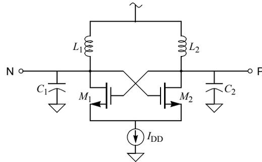
The procedure starts by using an RF simulator such as SpectreRF to compute the normalized phase noise  $L$ . Its PNoise analysis is used, with the *maxsideband* parameter set to at least 10 to adequately account for noise folding within the oscillator.<sup>12</sup> In this case,  $L = -110$  dBc at 100 kHz offset from the carrier. Apply (86) to compute  $c$  from  $L$ ,
