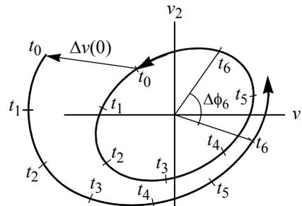
Since the oscillator is stable and the duration of the disturbance is finite, the deviation in amplitude eventually decays away and the oscillator returns to its stable orbit ( $\alpha(t) \rightarrow 0$  as  $t \rightarrow \infty$ ). In effect, there is a restoring force that tends to act against amplitude noise. This restoring force is a natural consequence of the nonlinear nature of the oscillator that acts to suppress amplitude variations.
