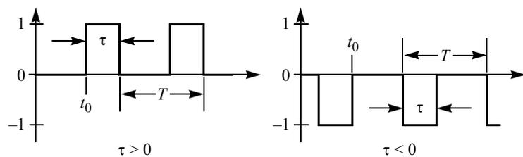
The input source produces a signal  $v_{in} = \Pi(t_0, T)$ . Since this is the input,  $t_0$  is arbitrary. As such, we are free to set its phase  $\phi$  to any value we like.
