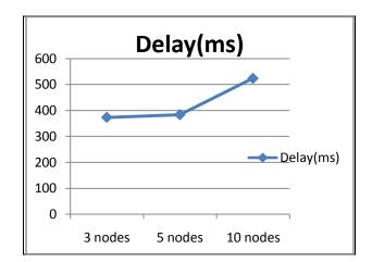
Fig3. Delay when AODV works normally
