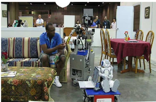
Figure 19. “Open Challenge” (Robocup@Home world competition, Singapore). Nono, a NAO-typed robot, discusses with “Daniel”, moves on OP-Y platform and then calls RH-Y, which brings drinks and snacks. Application developed and programmed in Piaget
