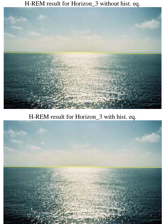
Figure 3. H-REM detection results for the Horizon_3 image with and without histogram equalization (hist. eq.). The horizon line is marked (in yellow). Note the error introduced in the top figure.
