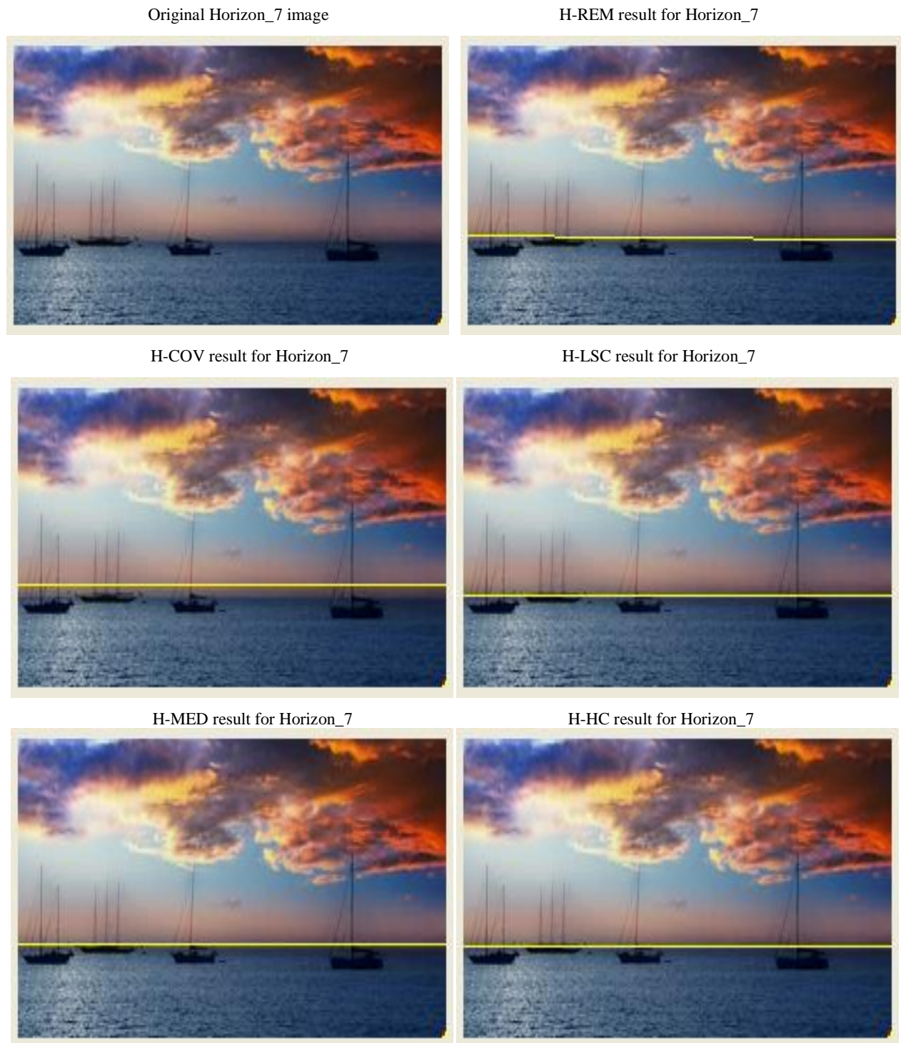
Figure 7. Horizon detection results for image Horizon_7. The (yellow) line marks the detected horizon. Note that a significant area of the image is covered by clouds introducing a challenge for correct horizon detection.
