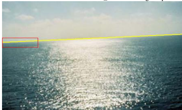
Figure 1. H-REM detection results for the rotated Horizon_3 image with and without (w.o.) filtering out of pixels. The horizon line is marked (in yellow). Note the error introduced in the top figure, especially in the area marked with the rectangular frame.
