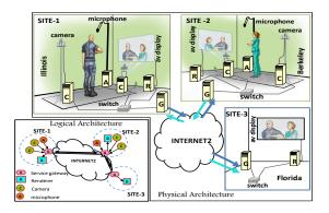
Figure 1: A 3D Tele-immersive Environment with Three Sites.
