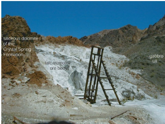
Figure 4. Site of the historic Pleasanton talc mine in Death Valley National Park, California, an example of the talc deposits of the southern Death Valley region (Wright, 1968; Van Gosen, Lowers, and Sutley, 2004; and Van Gosen et al., 2004b). The talc-tremolite rock formed through metasomatic reactions caused by the intrusion of the gabbro sill into the siliceous dolomite.
