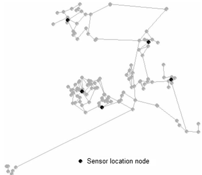
**Fig. 4.** Five sensor locations identified for Network 1 based on betweenness centrality, community structures, and graph distance
