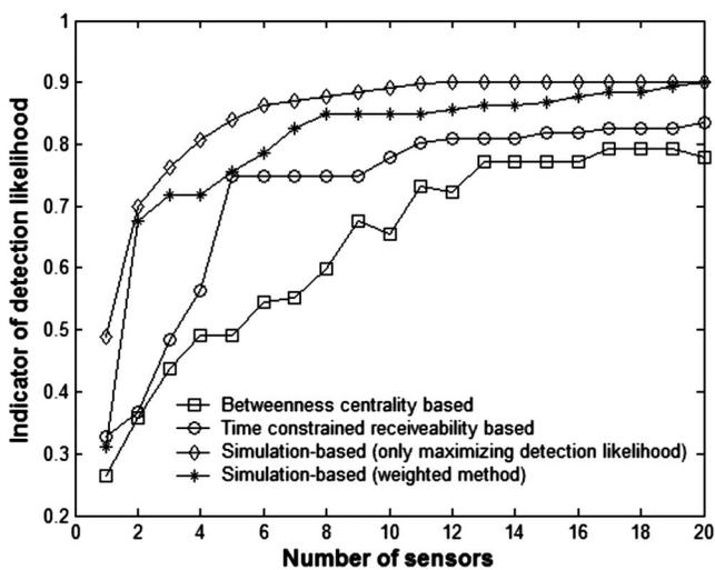
Fig. 10. Comparison of different sensor-placement schemes based on the detection-likelihood criterion
