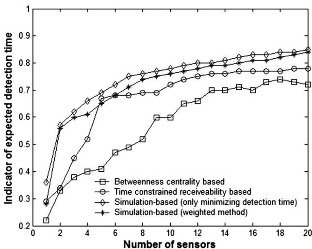
**Fig. 7.** Comparison of different sensor-placement schemes based on the expected-detection-time criterion
