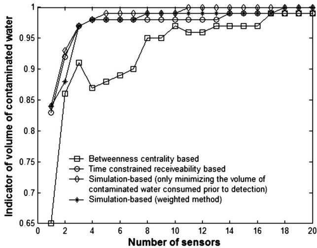
Fig. 9. Comparison of different sensor-placement schemes based on the expected-volume-of-contaminated-water-consumed criterion
