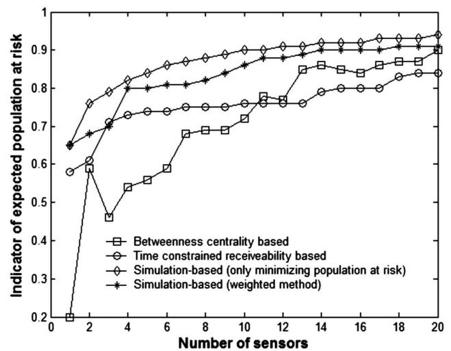
**Fig. 8.** Comparison of different sensor-placement schemes based on the expected-population-at-risk criterion
