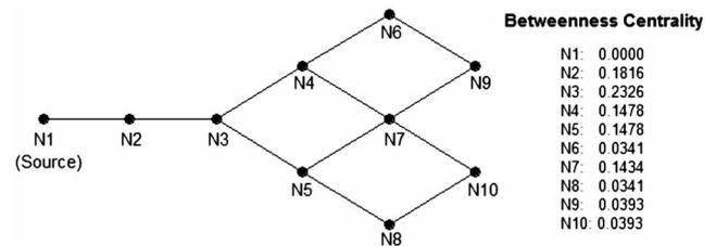
Fig. 1. Illustration of betweenness centrality with a hypothetical water distribution network
