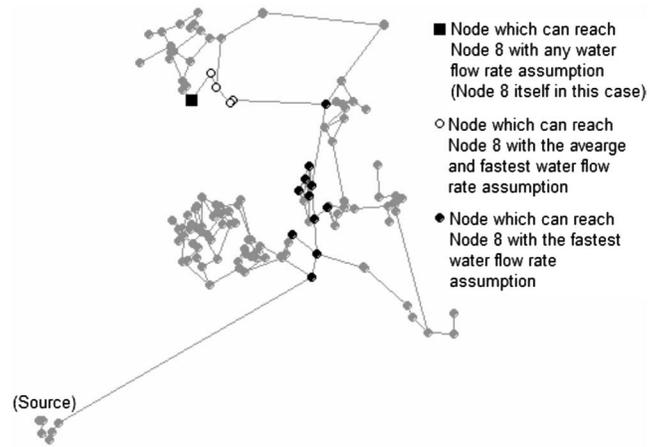
**Fig. 6.** Receivability for Node 8 under the time-constrained condition (150 min) with different water flow rate assumptions
